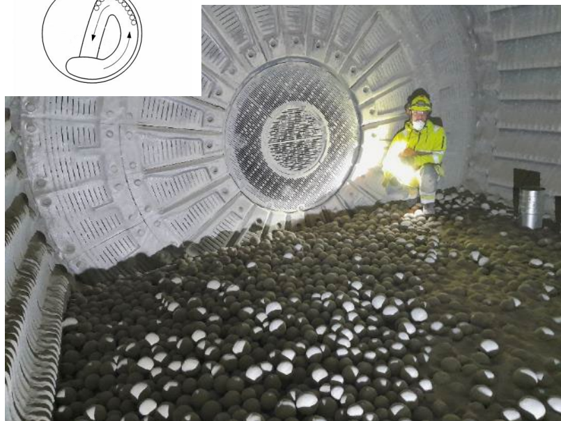
a) Cataracing of grinding media (Chamber 1)
