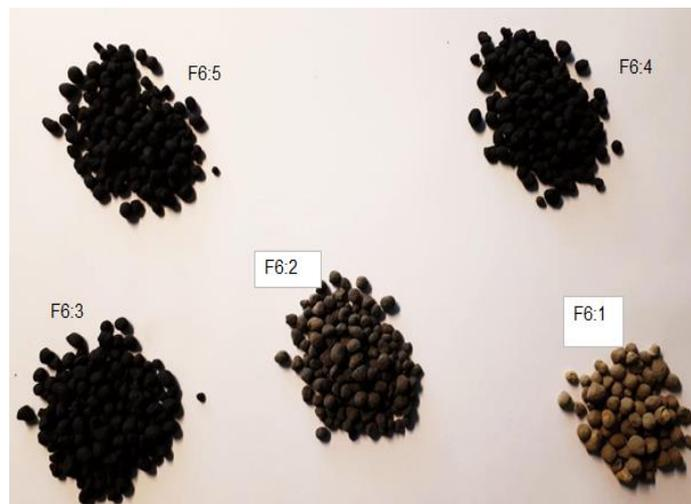
Figure 8. The heated raw meal nodules shown at various temperatures.
