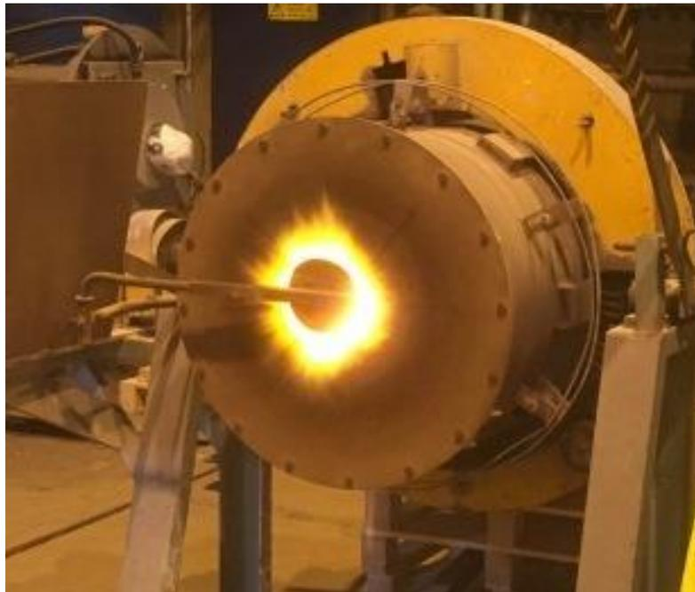
**Figure 6. Test configuration of plasma generator from ScanArc together with rotary batch kiln from Cements Research.**
